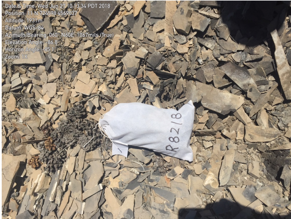
Figure 12. Photo of Sample No. R8218 which is a finely laminated, fetid black (unoxidized) mudstone (Table 5) with 3.5% P 2 O 5 .
